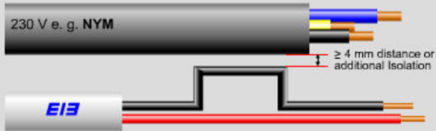
Isolated single core of the bus cable adjacent to the sheathed mains cable
