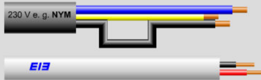
Isolated single core 230V adjacent to the sheath of the bus cable
